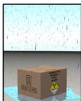
WATER Water spray for 1 hour to simulate rainfall of 2 inches per hour.
