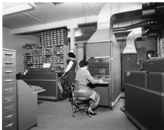
Computer Centre, 1958. Note the substantial ductwork necessary for air cooling of the vacuum tube processor. AUO-PHO-NB-32-11.
