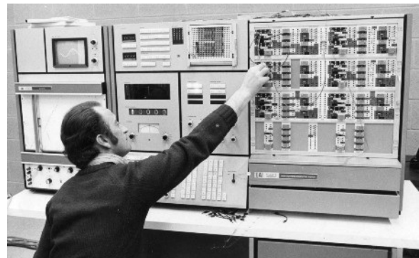
An analogue computer in use, ca. 1970. Analogue computers used electric circuit elements to simulate the dynamic behaviour of mechanical and other systems. AUO-CON-NB-6-1226-88
