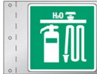
Fire hose cabinet with sprinkler floor valve
