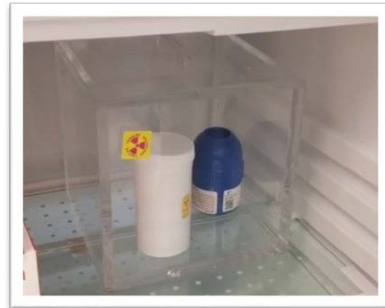
Shielding for sample storage
