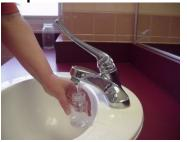
**Turn The Water Down** Do not flush out the powder. Allow 1" head space. **Do not** breath towards sample.
