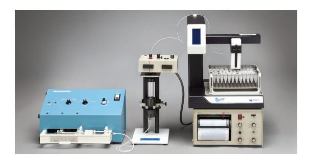
The system produces a continuous absorbance profile as the gradient is displaced from the bottom up by a dense chase solution and collected in precisely measured fractions.
