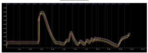
The trace overlay graphic editor allows for the comparison of multiple traces. This includes the ability to synchronize both the trace start times and the absorbance.
