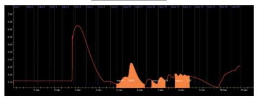
By using a simple drag of the mouse, specific regions can be highlighted and quantified (area under the curve). Multiple regions within a trace can also be defined. Further, the biometric editor allows for refining regions.
