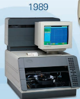
Dektak 8000 First Profiler with 3D Capability
