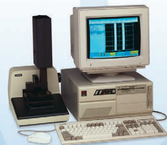
Dektak 3 First PC-Based Profiler
