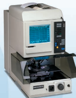
Dektak 3030 First Profiler for 150mm Wafers
