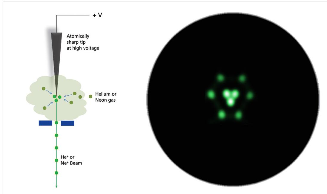
Image of the atoms at the end of the source tip emitting helium ions.
