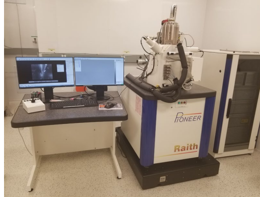
Raith Pioneer SEM + EBeam Electron-beam lithography and Scanning electron microscope
