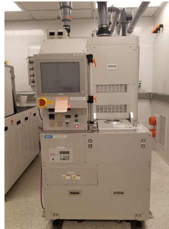
SAMCO RIE-110ip Etching System Inductively coupled plasma reactive ion etching (Si and III-V)
