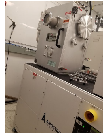
Angstrom Nexdep Evaporator Evaporation and chemical vapour deposition
