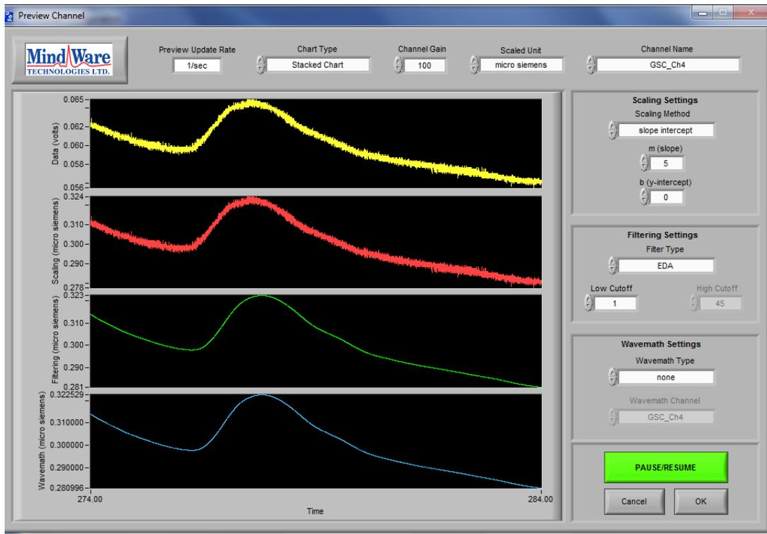
The yellow data line is thick and shows a lot of noise. Check the connections and reduce the channel gain if it set too high. If the signal is still too noisy, replaces the electrodes.
