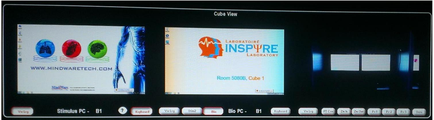
This window allows remote control of both computers (Stimulus PC and Bio PC) in the selected workstation and remote control of the workstation's camera.
