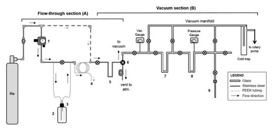
Figure 1 Schematic diagram of multipurpose line for extraction of waters (DIC/DOC) and  $CO_2$  (CX) samples, showing (A) flow-through section and (B) vacuum section. Numbers are described in the text.
